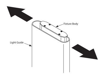
**Step 2:** Position one edge of the Light Guide inside the LED slot on one side of the fixture body.
